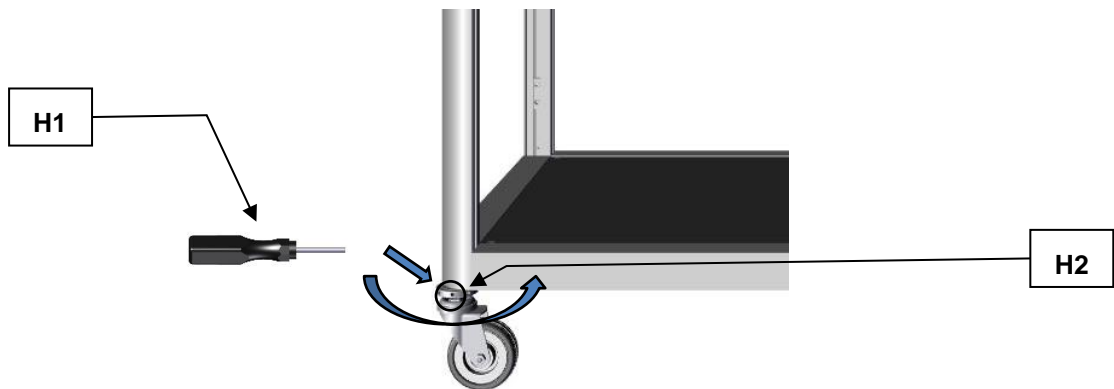
Fig. 5: Adjusting the height of the support structure
